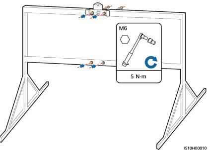
Figure 4-15 Securing the mounting bracket
