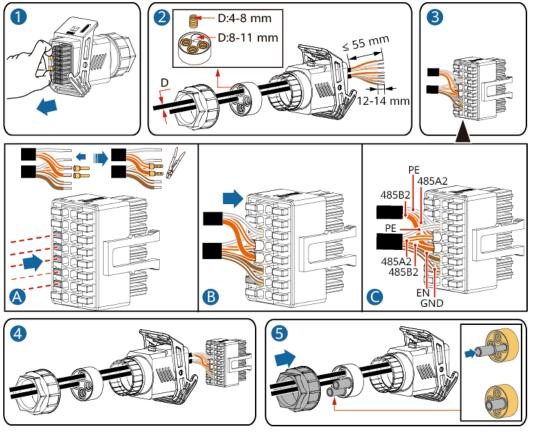
Figure 5-34 Installing the cable
