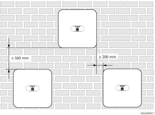
Figure 4-4 Staggered installation (recommended)
