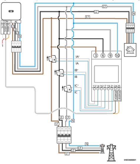
Figure 5-27 Three-phase, four-wire connection (Smart Dongle networking)
