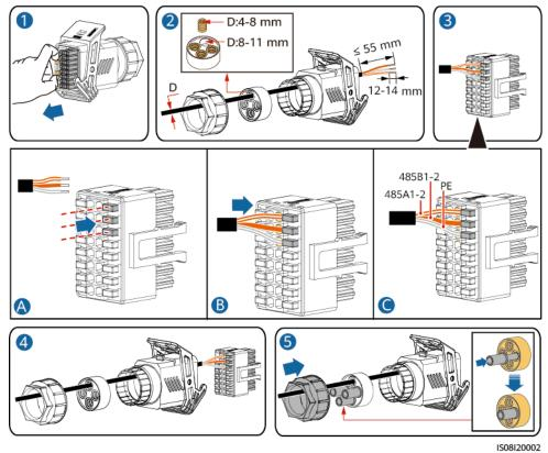
Figure 5-36 Installing the cable
