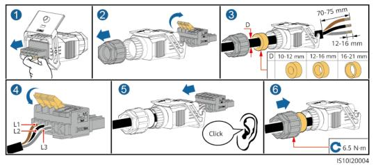
Figure 5-6 Four-core cable (L1, L2, L3, and PE)
