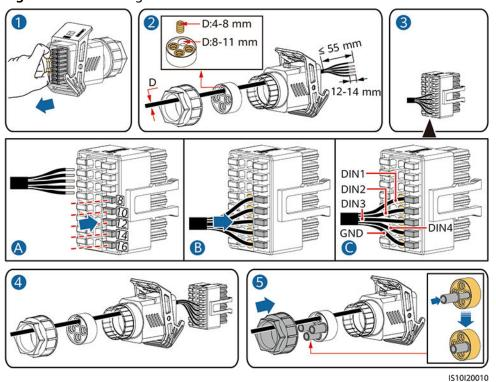
Figure 5-43 Installing the cable
