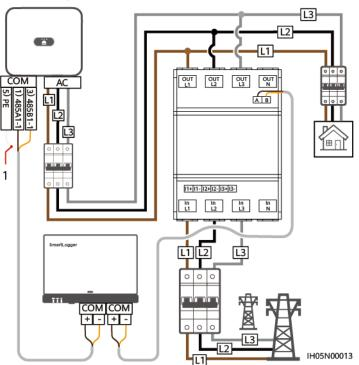
**Figure 5-30** Three-phase, three-wire direct connection (SmartLogger networking)
