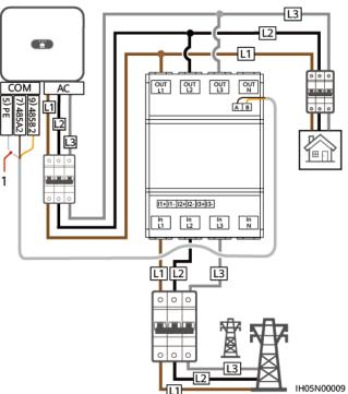
**Figure 5-28** Three-phase, three-wire direct connection (Smart Dongle networking)
