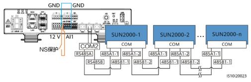
Figure 5-50 Connecting the SmartLogger to the NS protection switch
