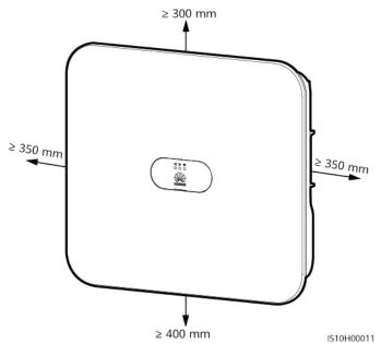
• When installing multiple SUN2000s, install them in horizontal mode if sufficient space is available and install them in triangle mode if no sufficient space is available. Stacked installation is not recommended.
